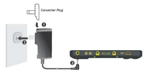
3. The charge indicator glows in amber when charging is in progress. Do not disconnect your device from AC power until the battery is fully charged, as indicated by the amber indicator turning into green. This will take a couple of hours.
