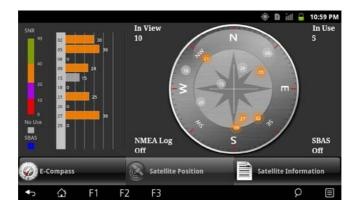
SBAS (satellite-based augmentation system) provides additional accuracy and reliability for the GPS devices. Ground stations are necessary to achieve the purpose. The SBAS feature works where such stations exist. You can enable the SBAS feature. (See "Getac Peripheral Settings" in Chapter 9.)
