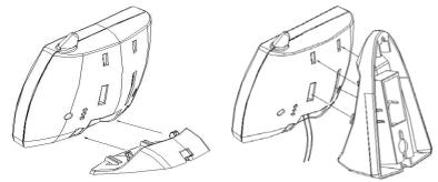
Connect the telephone line cord to the telephone jack, and the power supply to a live power outlet. Make sure you are not using an outlet controlled by a switch.
