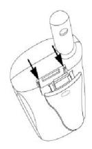
Hook the belt clip into the notch at top of the radio and slide down until it clicks into place.
