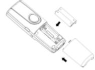
Insert two pieces AAA batteries in the compartment, ensuring correct polarity and close the compartment.
