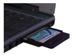
• Push it in firmly and ensure it is seated properly. Only the thicker portion will protrude from the slot.
