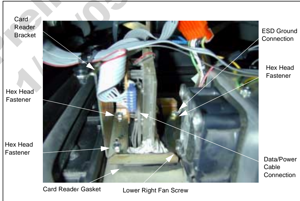
Figure 11: Top View of Card Reader Mounted In Option Door
