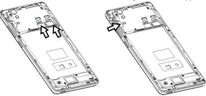
3. Finally insert the battery and replace the rear cover of the mobile phone.
