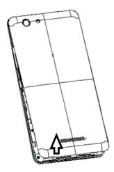
2. Remove the battery and insert the Micro SIM and SD cards to the card slots correctly.
