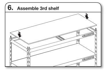
Repeat steps 1 and 2. We recommend adding a section at notch 14 from the bottom of the post. Add the horizontal and side support beams. Add tie channel support and shelf.
