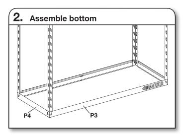
Repeat step 1 to assemble the other three corners, completing the bottom shelf. Make sure to press firmly on all side and horizontal support beams (P3 and P4) to ensure they are properly installed in the top and bottom posts.
