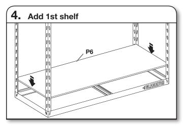
Add laminate shelf to the bottom of the frame. Gently place laminate shelf on beams and tie channel support.
