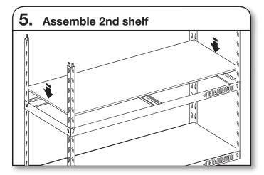
Repeat steps 1 and 2. We recommend adding a section at notch 8 from the bottom of the post. Add the horizontal and side support beams. Add tie channel support and shelf.
