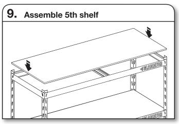
Repeat steps 1 and 2. We recommend adding section at the top of the post. Add the horizontal and side support beams. Add tie channel support and shelf.
