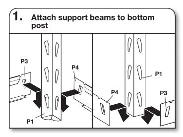
Use the bottom post (P1) and attach a horizontal support beam (P3) across front, and attach a side support beam (P4) to the other side. Insert horizontal and side beams starting at the top of the slots on the upright posts and pushing down after engagement. This will give you support while building your shelves up. You have now assembled one corner.
