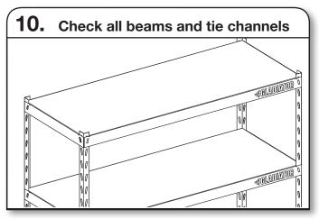
Verify that all beams and tie channel supports are properly assembled and firmly seated into the top and bottom post slots.
