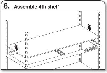
Repeat steps 1 and 2. We recommend adding a section at notch 8 from the top of the post. Add the horizontal and side support beams. Add tie channel support and shelf.
