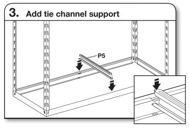
Add tie channel support (P5) to the bottom of the frame. Rotate into place BEFORE dropping tabs in slot.
