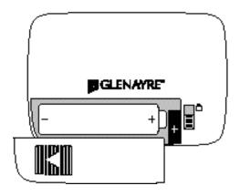
CAUTION: Be careful to align the + and - symbols on the battery with those inside the battery compartment. Inserting the battery backwards will cause the date and time setting in your AccessLink II pager to be lost. All messages will be preserved, however.
