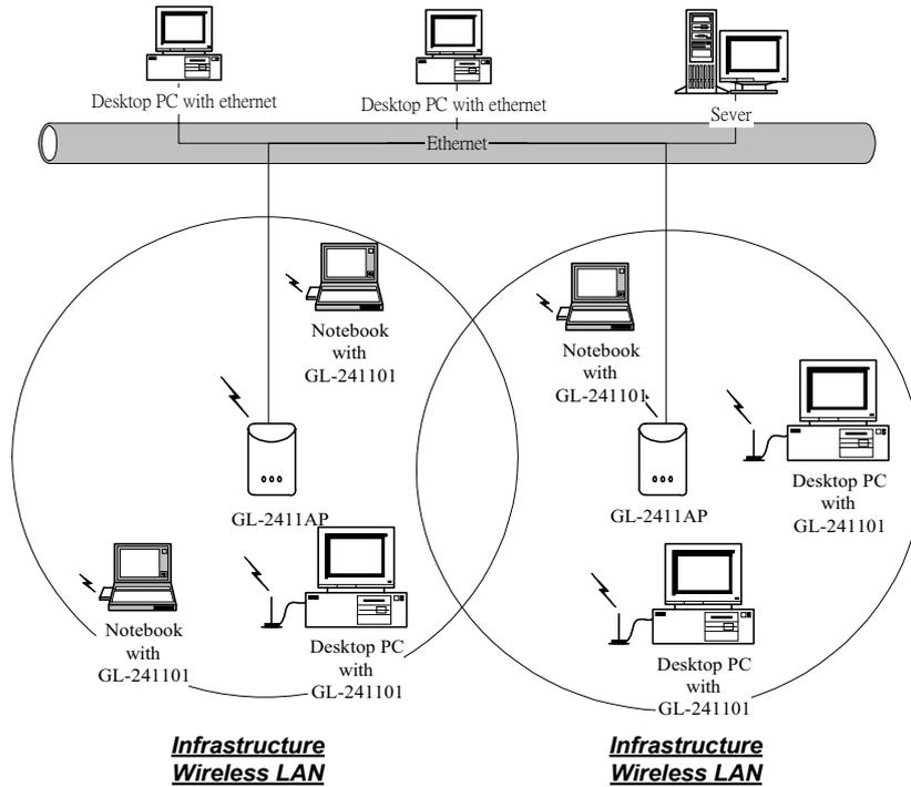
**Fig. 2 - Infrastructure Wireless LAN Configuration**
