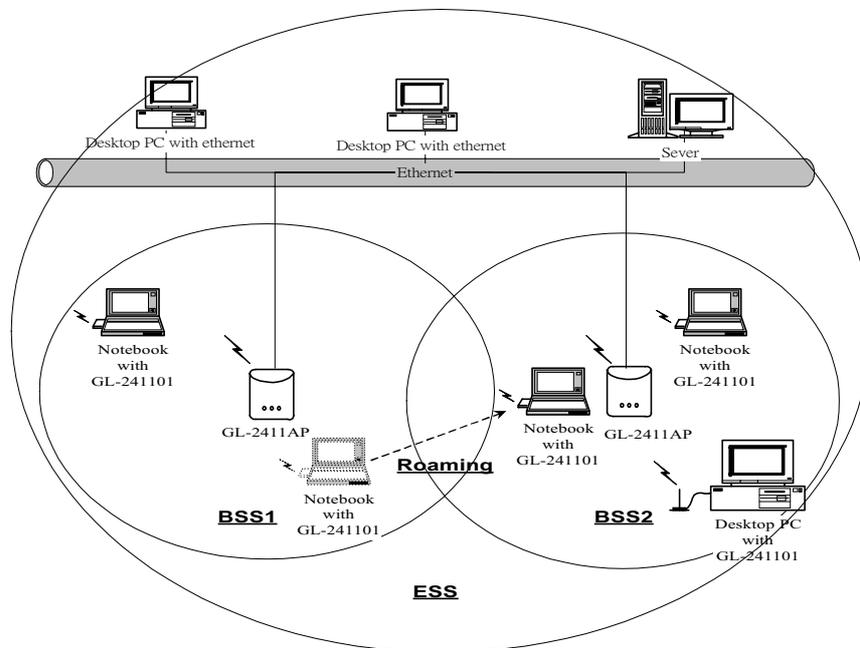
Fig. 4 - Roaming in an Extended Service Set (ESS)
