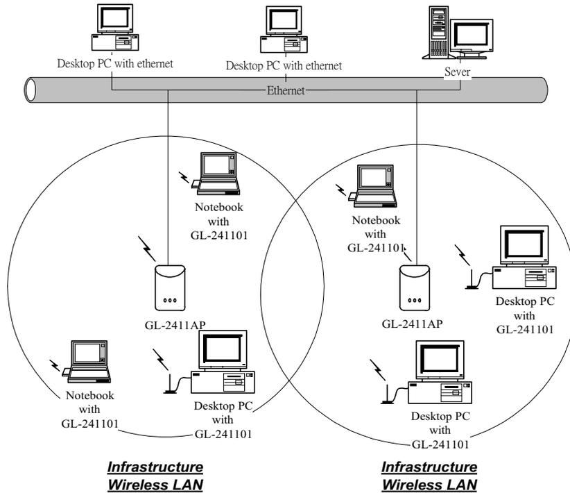
**Fig. 2 - Infrastructure Wireless LAN Configuration**
