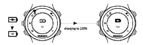
When you connect the watch to a power source, the watch will turn on in charging screen. Charge the watch until the battery icon stays still as above.
