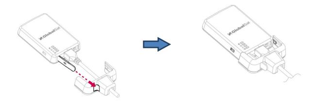
Using the device for the first time, rechargeable battery will require a complete 100% charge before LT-501/LT-601 is operable. To maximize your device's battery life, proceed by performing the steps listed below.
