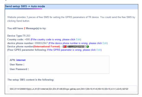
Free web service provides 3 pieces of free SMS for configuring TR-203A. If you want to change the configuration after sending 3 pieces of free SMS, please go to **Setup > Send Setup SMS> Manual Mode**.
