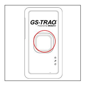
Shortly press the emergency button to make TR-203A connect to Free Web Service.
