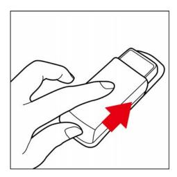
After putting TR-203A in the carry bag, you could take out it by pressing on the bottom of the bag and pushing outward TR-203A according to the direction on the picture. Belt clips, holsters and similar accessories, other than the approved accessory for this product, may only be used if the assembly does not have a metallic component.
