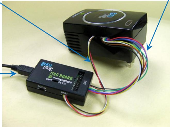
This is the standard 20pin JTAG connector which has the same pin signals as 8 pin cable
