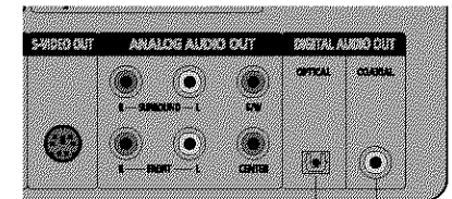
To Digital Audio Input of an A/V Receiver with a Dolby Digital Decoder
