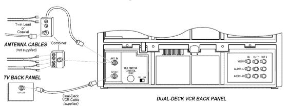
If you have separate VHF and UHF antennas, you will need to purchase a device called a combiner. This attaches to both antenna cables on one side and to a cable which goes to the VCR's ANT IN connection on the other.
