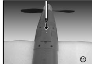
11. Installed by Screw \phi 2.0 \times 6PB
