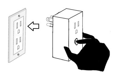
After 3 seconds, release the button. If you see the button blinks, that means the module has been reset successfully and you may retry Step 3 above to add the module into your network.
