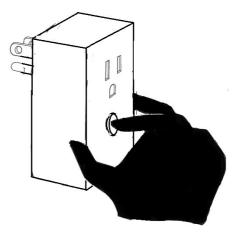
c. Plug the module back into the AC outlet with the button pressed
