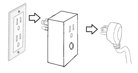
b. Press and hold the button on the module
