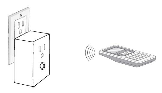
Once the PA-100 has been added to your network, you may assign it to a Group or Scene, change its status when the All ON or OFF command is received from the controller. It can also be set in Association with another Z-Wave device to perform a specific duty. Please refer to the instructions manual of your gateway or remote controller for detail procedures on how these functions can be set.
