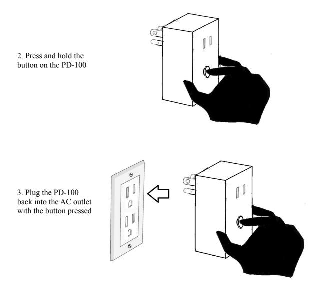
After 3 seconds, release the button. If you see the button blinks, that means that the PD-100 has been reset successfully and you may retry Step 3 above to add the module into your network. Otherwise, please repeat the manual reset procedures.
