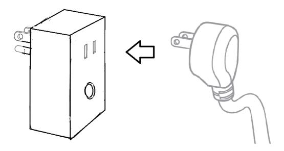
Step 2. Insert the module's 3-pin plug into an AC outlet of your preferred location. In normal operating mode, the LED on the front panel will be lit.
