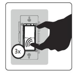
If you see the lighting turns OFF, it means that the module has been reset successfully and you may retry Step. 5 above to add the module into your network. Otherwise, please repeat the manual reset procedures.
