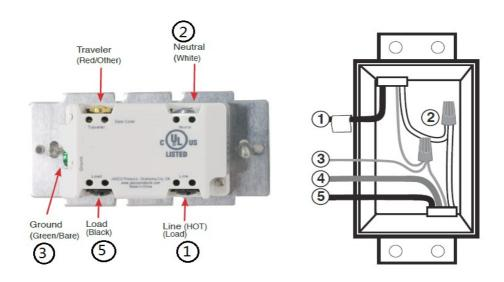
The Traveler terminal is not used in a 2-way circuit. Do not remove the insulation tape on the Traveler terminal in this application
