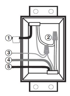
4 wires for 2-way circuit
