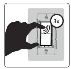
Then, quickly tap the bottom side(OFF) of the rocker 3 times
