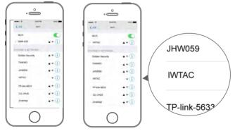
Fourthly, after successfully connect iPhone with IWTAC, users now can operate APP, enter WiFi name and password . Click "Connecting", then panel and APP enter bonding process.
