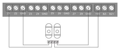
Note: For wired beams detector, its power consumption is a little large, so if install over than 2 pairs beams, need to use external power supply.
