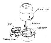
Use a Philips head screwdriver to detach the car from the battery cover and pedestal.
