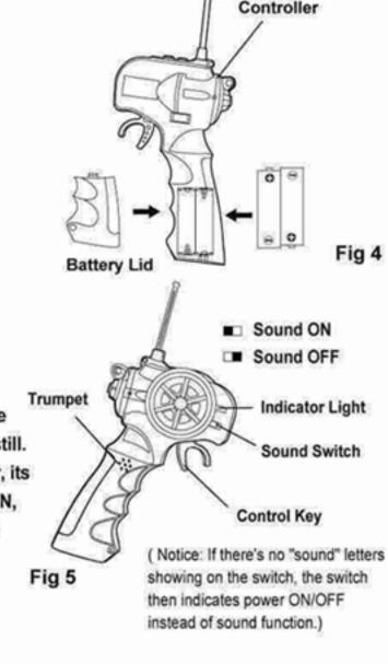
4) Push the control key on the controller slightly upward, the car will move backward, if push the control key to the very end, the car will reach to its top speed. Slightly pull the control key backward, the car will move forward, if pull it to the very end, the car will reach to its top speed. (Fig 6)
