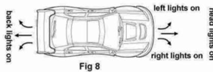
5) When pushing or pulling the control key, turn the revolver button clockwise at the same time, the car will turn right forward or right backward. While turn the revolver button anticlockwise, the car will turn left forward or left backward. (Fig 6,7,8)
