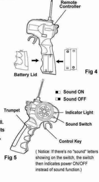
4) Push the control key on the controller slightly upward, the car will move backward, if push the control key to the very end, the car will reach to its top speed. Slightly pull the control key backward, the car will move forward, if pull it to the very end, the car will reach to its top speed. (Fig 6)
