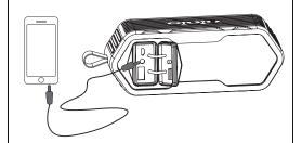
3, Changing: when charging, an orange LED light will illuminate. The orange light will turn off when your unit is fully charged
