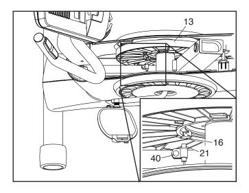
Turn the Pulley (13) for a moment. If necessary, repeat the step above until the console displays correct feedback.
