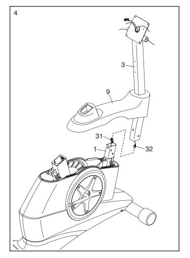
5. **Tip: Avoid pinching the wires.** Slide the Upright (3) onto the Frame (1).
