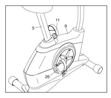
Using a flat screwdriver, release the tabs along the bottom edge of the Top Shield (9) and slide the Top Shield upward. Then, using an adjustable wrench, turn the Right Pedal (26) counterclockwise and remove it.
