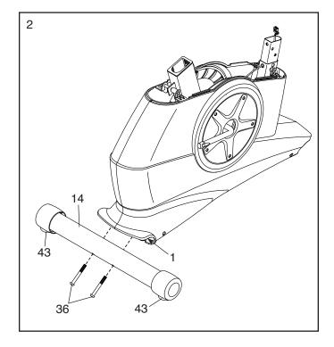
Set a sturdy piece of packing material under the front of the Frame (1). Have a second person hold the Frame to prevent it from tipping while you complete this step.
