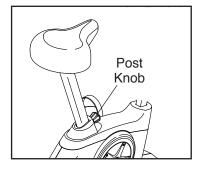
adjustment holes in the seat post. Move the seat post upward or downward slightly to make sure that the knob is engaged in one of the adjustment holes in the seat post. Then, tighten the knob.
