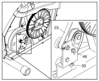
When the Drive Belt (23) is tight, tighten the M6 x 20mm Hex Screw (46).
