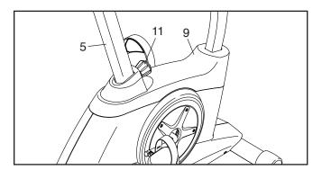
Using a flat screwdriver, release the tabs along the bottom edge of the Top Shield (9) and slide the Top Shield upward.
