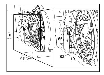
When the Drive Belt (19) is tight, tighten the M8 x 18mm Flat Head Screw (65).
