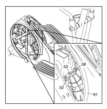
Next, rotate the Pulley (61) until a Magnet (58) is aligned with the Reed Switch (53). Slide the Reed Switch slightly toward or away from the Magnet. Then, retighten the M4 x 16mm Screw (52). Rotate the Pulley for a moment.
