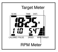
As the target meter changes in height during the workout, adjust your pedaling speed so that the same number of bars appears in both meters. If your pedaling speed is slower than the current target speed, an arrow will appear next to the RPM meter to prompt you to increase your speed; if your pedaling speed is faster than the target speed, an arrow will prompt you to decrease your speed.
