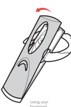
Using your fingernail, carefully prise open the fascia shell from the back of the headset upwards and forwards.
