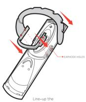
Line-up the earhook holes with the pins and gently guide the replacement earhook over the top until set in position.
