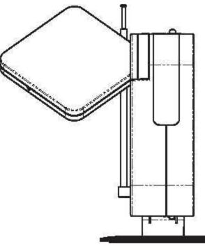
Option 1- Surface mounting (horizontal) using snap on anti-slip base.
