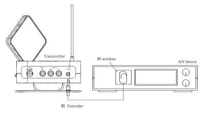
Controlling the A/V device remotely with your remote control: Operate the A/V source's remote control (the A/V device that is connected to the transmitter) as you normally do while pointing it at the receiver. The receiver wirelessly sends the infrared command to the transmitter which then transmits it via the IR extender to the A/V source device.
