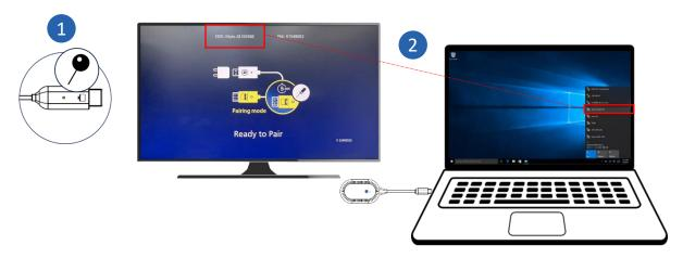
3) When the connectivity is completed, open the device's web browser and enter the IP address "192.168.203.1" into the settings page.
