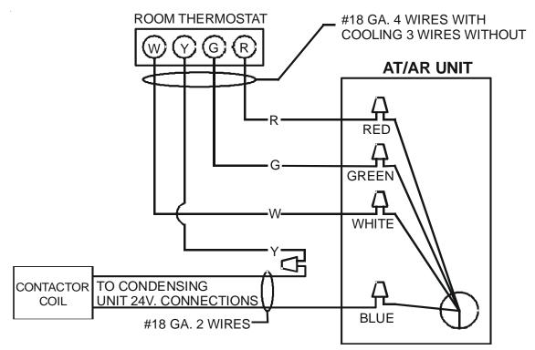
Figure 8 - Low Voltage Wiring Diagram for Cooling Unit with optional heat kit 10kW and below
