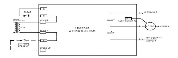
The Electronic Blower Time Delay Relay provides power to the blower motor with a delay of 7 seconds after 24VAC is applied to "G". After 24VAC is removed from "G", the blower motor output is de-energized after a delay of 65 seconds.
