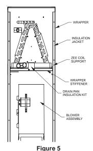
**NOTE:** When converted to downflow position, the coil may protrude above the cabinet on some models.
