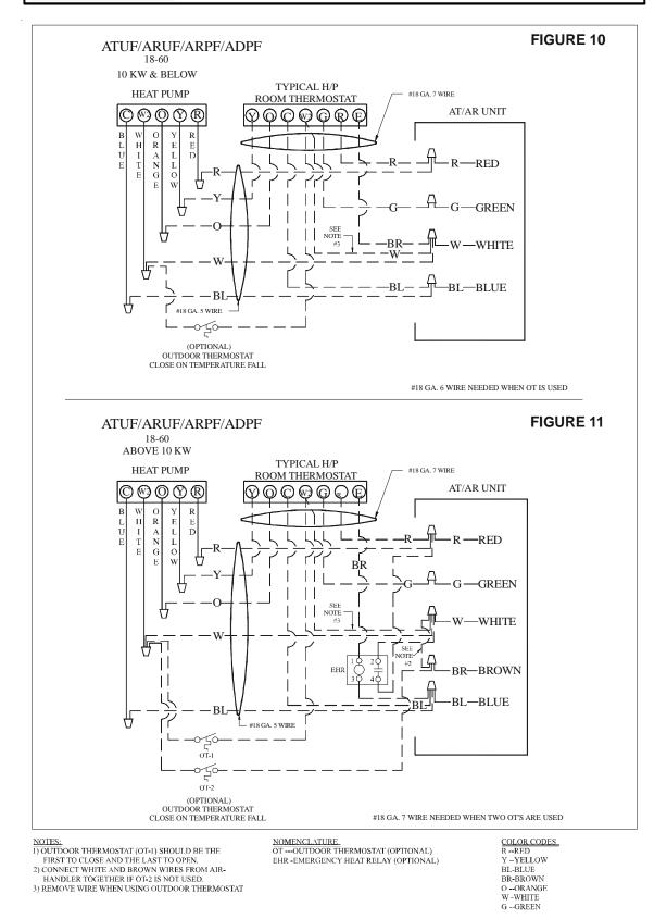
**IMPORTANT:** If outdoor thermostat is not used, tie white and brown wires from Air Handler together.
