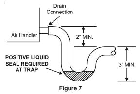
Use of a condensate removal pump is permitted when necessary. This condensate pump should have provisions for shutting off the control voltage should a blocked drain occur. A trap must be installed between the unit and the condensate pump.
