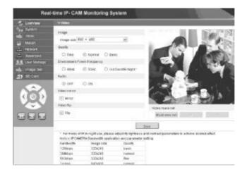
[Image size]: Used to set the resolution of images. You may select a resolution of coding formats VGA (640\*480) and QVGA (320\*240).
