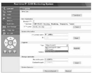
The interface forsetting **System** parameters of the IP Camera is shown in the above figure. You may set the time, name, upgrade page, and capturing/recording path of the IP Camera.
