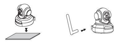
5-2-2 Suspended installation: There is a 1/4-inch screwhole on the bottom of the IP Camera. The user canbuy a metal plate or metal bracket for installation according to actual needs
