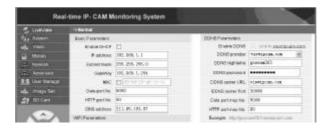
Please select **DDNS provider**, for example, **viewipcam.com**. Enter the DDNS logon name and logon password, for example, **goscam003**, and adopt default values for other parameters. Click <Apply> and the IP Camera will reboot. After re-connection, you will view that the "current operation status" changes to "updating IP address and DDNS server successfully". It indicates the DDNS setting succeeds.
