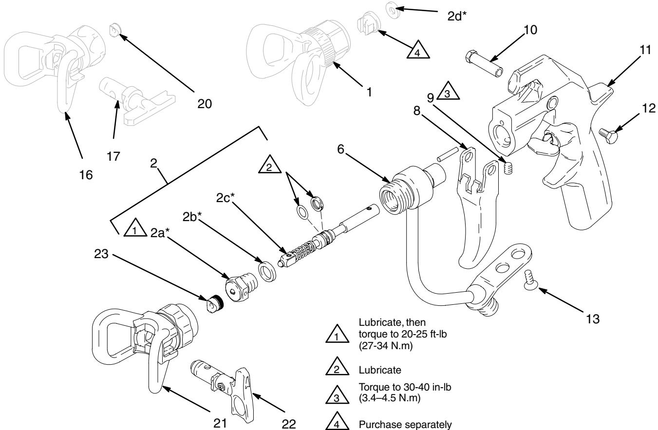
**235460, C:** Standard (non-reversing) DripLess™ Tip Guard; 2-finger trigger. *Includes items 1 to 15*
