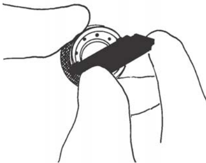
FIG. 27: Unthread Cap from PCD Body
