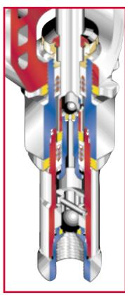
Long Lasting Packings Ultra high, molecular weight, polyethylene design
