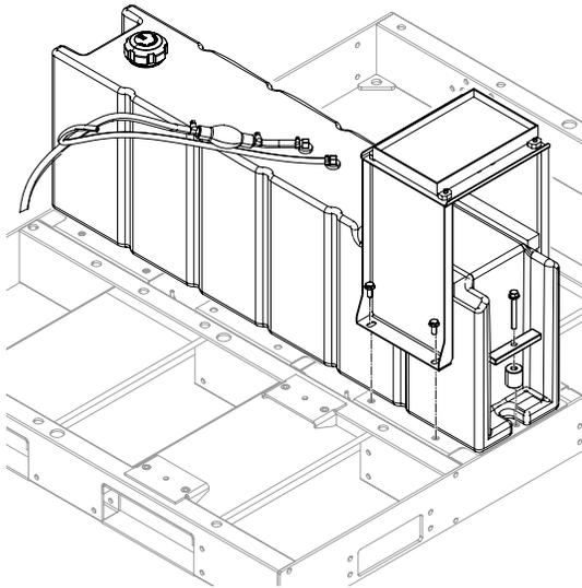
Remove Battery Bracket and Fuel Tank
