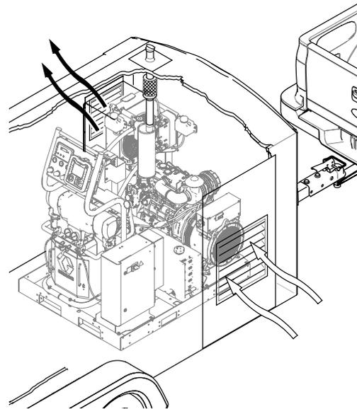
Radiator Exhaust and Air Intake Louvers
