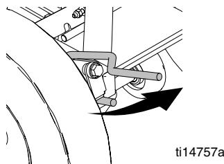
4. Slide Engine Throttle Lever (A) to desired setting.
