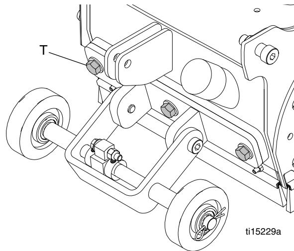
4. Adjust plate until guide wheels lay flat on surface.
