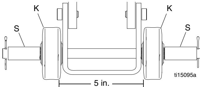
To make a **10 in. cut**, install two spacers (S) on **inside** of Depth Control Wheels (K).
