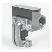
Cycle Indicator Switch (SPDT): Used in conjunction with the cycle indicator pin at cycle rates not exceeding 60 cpm, it provides an electrical signal to the system controller which counts cycles to monitor and verify completion of the lube cycle. Part number: 563272 (510-599-000). A moisture-resistant switch, 563273 (510-599-200), is also available.
