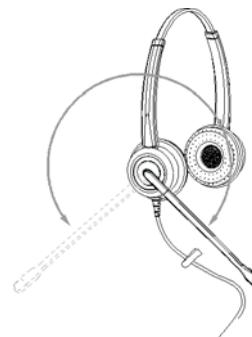
The GU3000 can be worn on the left or right by flipping the microphone to the other side (300° limit). To change ears, rotate the microphone boom over the headband to accommodate the left or right ear.
