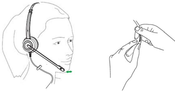
To avoid low or distorted sound, and to provide clear and crisp telephone calls, the microphone should be positioned within 30-40mm of your mouth. The microphone boom arm will move in a variety of directions to ensure the best fit.
