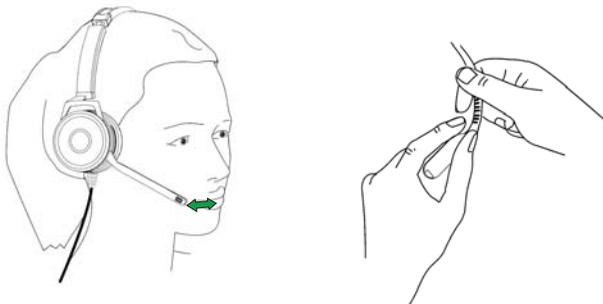
To avoid low or distorted sound, and to provide clear and crisp telephone calls, the microphone should be positioned within 0.5 inches of your mouth. The microphone boom arm will move in a variety of directions to ensure the best fit.
