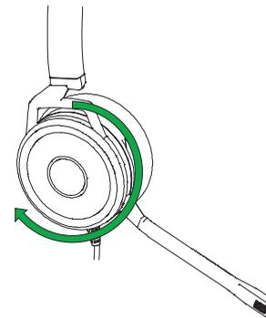
The GU3005 can be worn on the left or right by flipping the microphone to the other side (270° limit). To change ears, rotate the microphone boom over the headband to accommodate the left or right ear.
