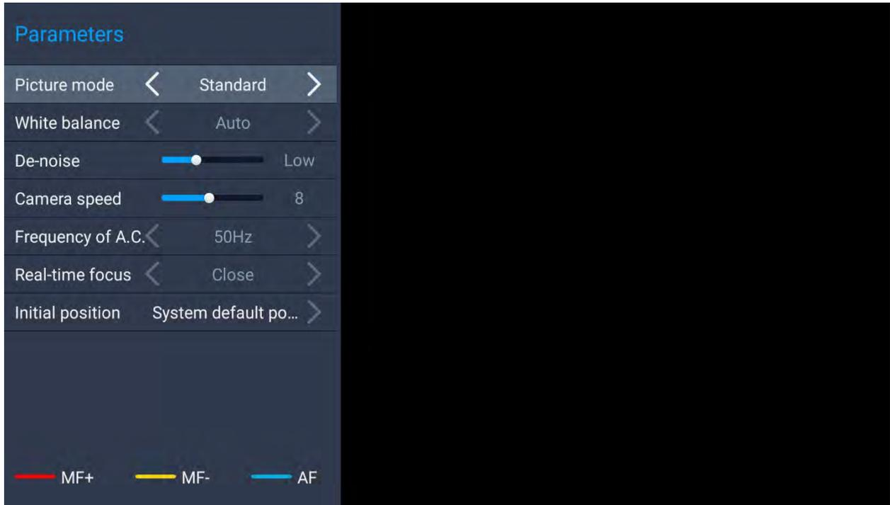
Figure 43: GVC3220 Camera Parameters Setting Screen
