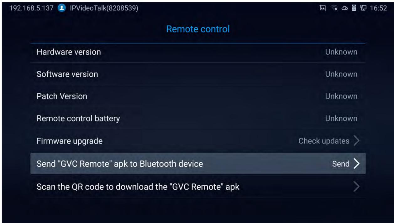
**Figure 81: Send the GVC Remote apk using Bluetooth**
