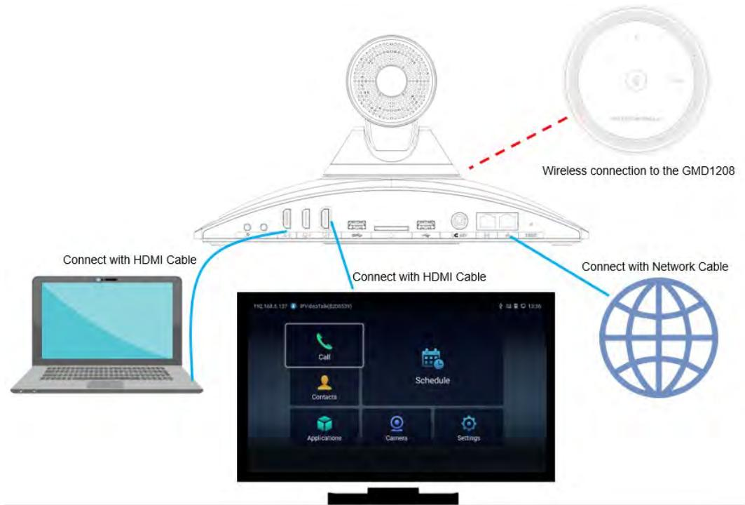
Figure 3: GVC3220 Back Panel Connection Diagram
