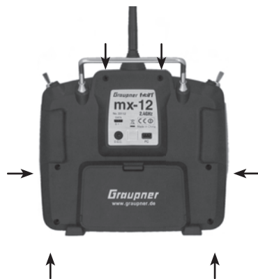
Arrangement of the case back screws
