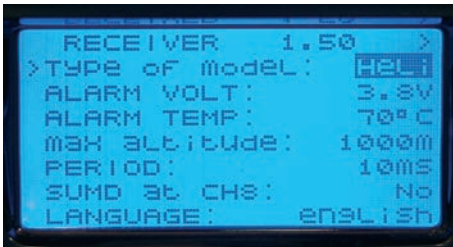
When opening the telemetry menu of a Graupner transmitter you have access to the receiver/SAS units, after switching to 'Heli' you are in the 'Base Setup...'
