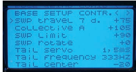
'Base Setup Control' scrolls through the initial model parameters
