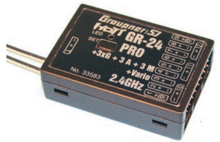
The GR-24 Pro serves 12 servos and external telemetry sensors can be plugged in
