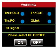
When you switch on the transmitter the position of the servos connected to the outputs 1 (plane) and 6 (heli) are checked. If the servo position is out of the idle range, the RF module will remain Off.
