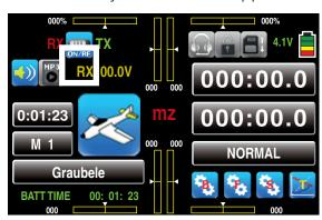
The red "RX" and green "TX" on the left and right of this switch symbol mean that the currently active model memory has once been linked to a *Graupner*-HoTT receiver but is presently not linked.
