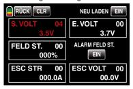
The transmitter battery voltage should be monitored in the LCD display during operation. Once the adjustable voltage in the "battery warning threshold" is reached in the "Etc.Set" submenu of the system menu, Seite 202, a standard 4.8 V (NiMH) for the mz-18 HoTT transmitter and 3.6 V (lith.) for the mz-24 HoTT transmitter, a warning beep sounds, and the following window appears in the display:
