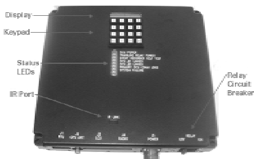
Figure 2.2-1 Setup Control Unit (SCU)
