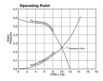
The operating point of the fan and the system is the point where these two curves intersect. This intersection will determine the cfm and Ps delivered.
