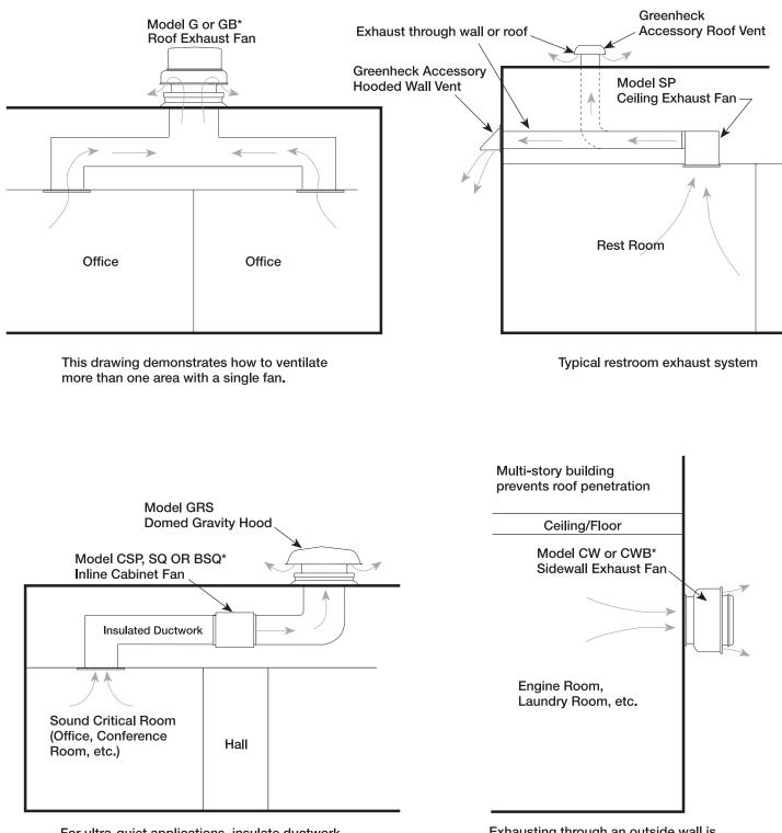
For ultra-quiet applications, insulate ductwork and mount fan over a less sound critical area.
