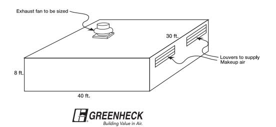
$\frac{9600 \text{ ft}^3}{4 \text{ min.}} = 2400 \text{ cfm}$
