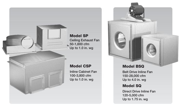
Models SP and CSP are designed for exhausting relatively clean air at temperatures up to 110°F. Motors are in the airstream. All models are direct drive and can be used with a speed control.
