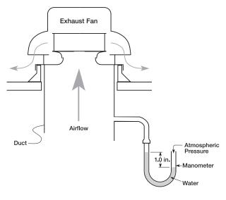
The amount of static pressure that the fan must overcome depends on the air velocity in the ductwork, the number of duct turns (and other resistive elements), and the duct length. For properly designed systems with sufficient make-up air, the guide lines in the table below can be used for estimating static pressure:
