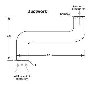
To calculate the system losses, one must know the ductwork system configuration (see Ductwork figure).
