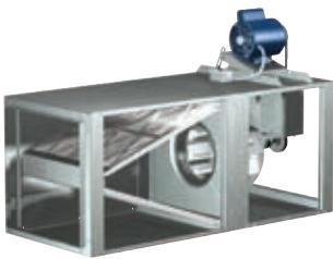
The filter box is designed to provide a compact and convenient clean air solution. Factory assembled as a single unit, this fan eliminates the costly process of designing, fabricating, and installing special remote filter box assemblies. Both the fan and filter section feature removable access panels on both sides to remove and replace filters, making fan maintenance simple and fast.
