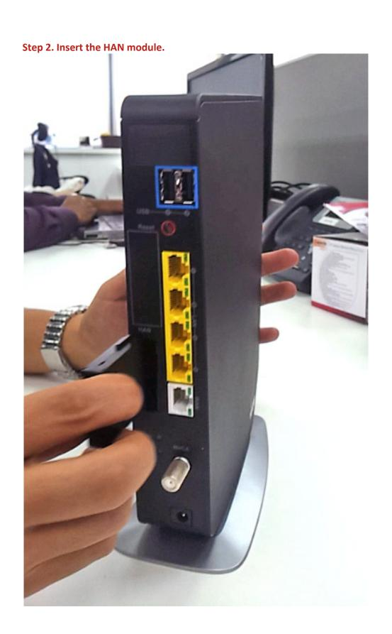
It can only go in with one orientation. It should slide in and come to a smooth stop with only the extraction finger handle protruding. If the module doesn't slide in very easy then verify that you have it the right way up. The HAN module label faces to the RIGHT when you watch the FiOS-BHR4 gateway from behind.
